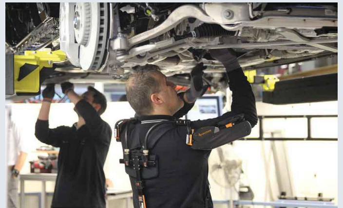
Figure 11: Overhead Exoskeleton Airframe made mandatory PPE by Toyota Motor NA
