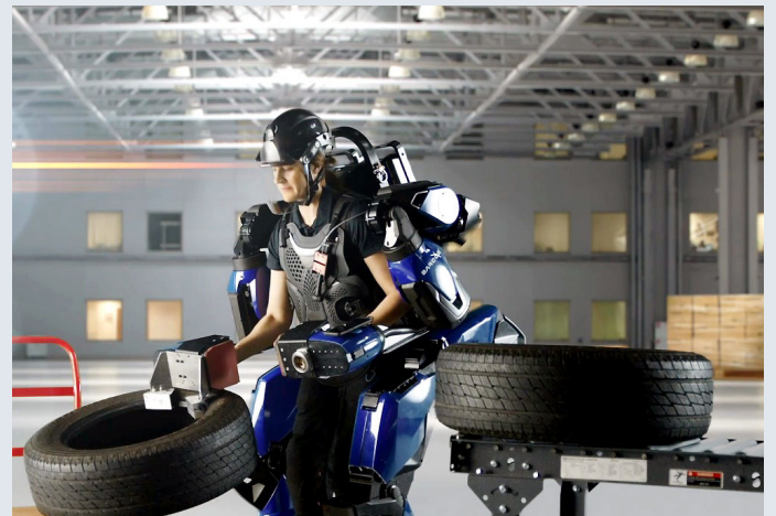
Figure 2: Sarcos' Guardian XO exoskeleton provides enhanced strength
